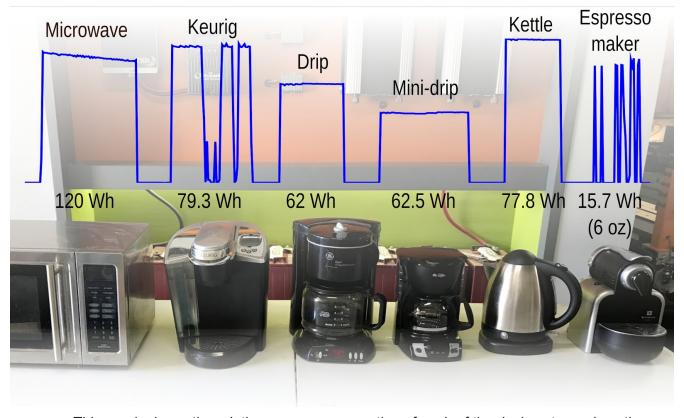
This graph shows the relative energy consumption of each of the devices to produce three servings of coffee, totaling 24 oz for all except for the espresso maker which made three two ounce shots. The area under each of those curves is the total energy consumed. Look at that huge chunk under the microwave curve!
